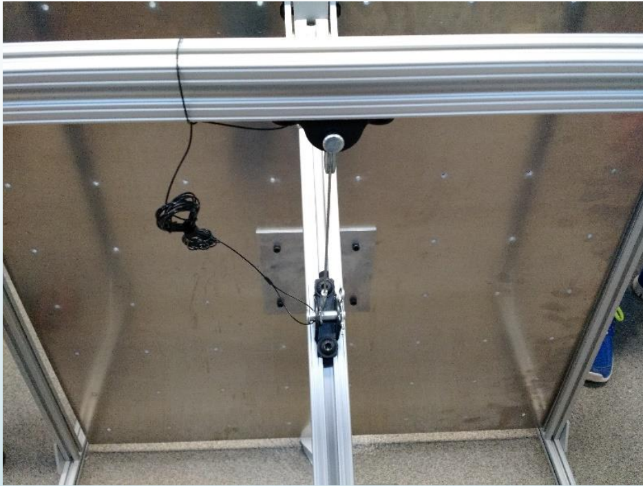
Lanyard with quick release pull pin attached to the T-slotted aluminum swing arm
