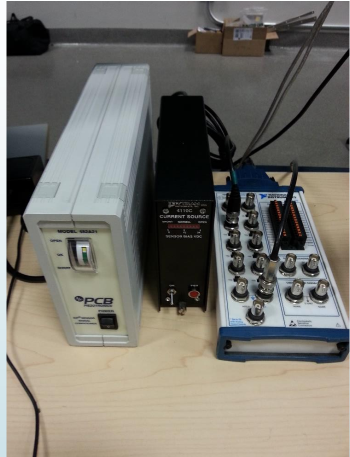
Initial data acquisition setup vs current setup with signal conditioner
