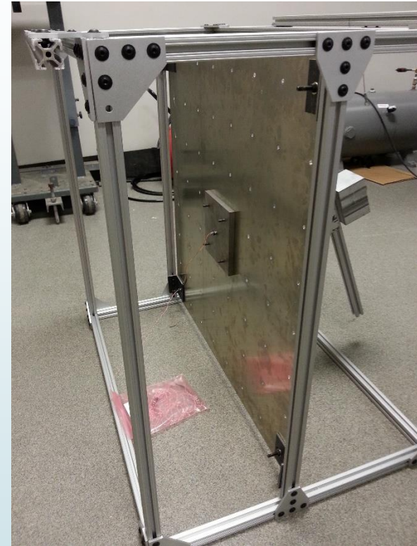
Back Side of Fixture Plate Showing Test Article Centered
